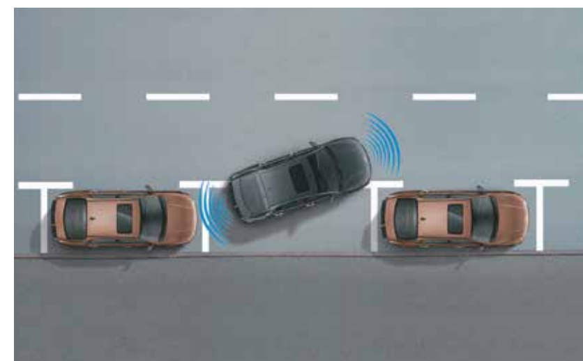
Parking assist (front & rear parking sensors and rear camera with dynamic guidelines)
