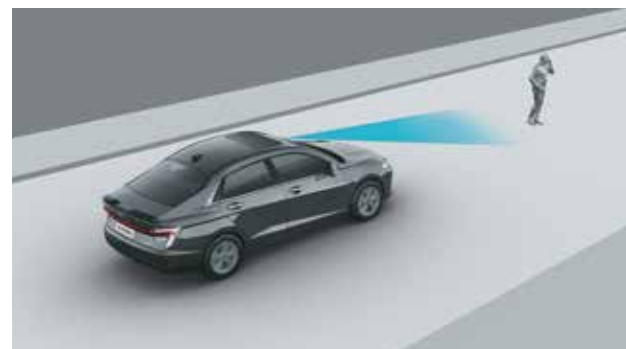
Forward Collision - Avoidance Assist - Pedestrian (FCA-Ped)
