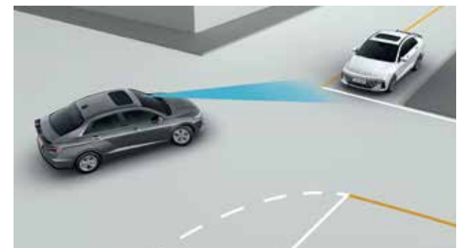
Forward Collision - Avoidance Assist - Junction Turning (FCA-JT)
